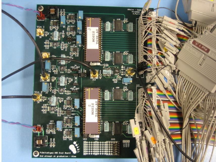
Figure 5.15: Fabricated PC board configured to test two custom designed chips in parallel.
