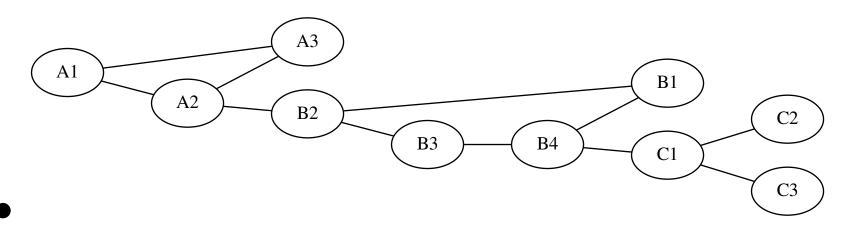
Packet A1 - A3 internal A1 - B2 goes to border router and across, then local A1 - C2 goes to border router to B network, across local to B/C border, then finally to C
