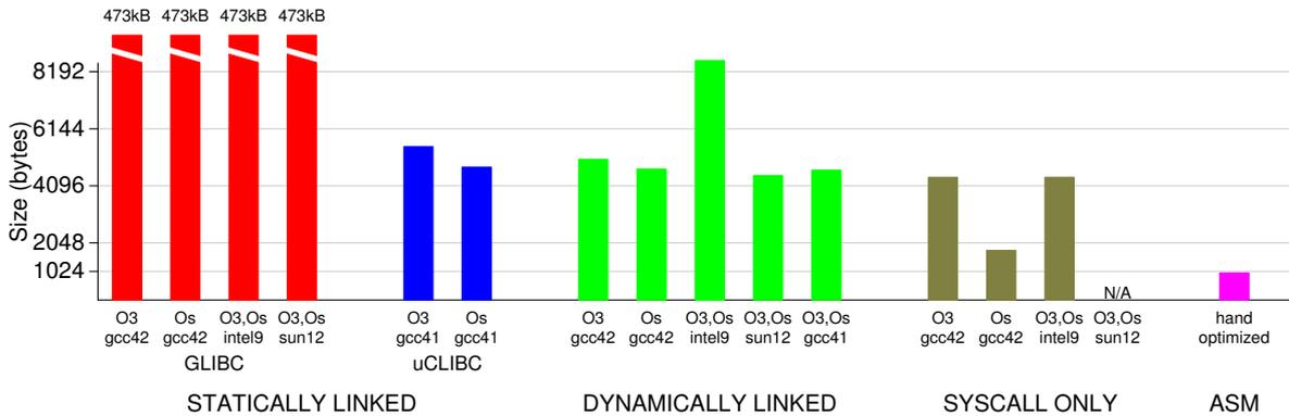
Fig. 7. Total size of generated executables, stripped of debugging information.
