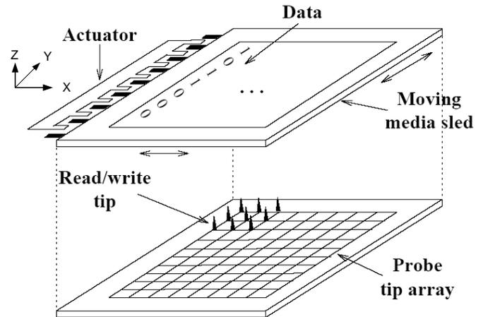
**Figure 1: A high-level diagram of a MEMS-based storage chip [8]. Every side of the media sled has an actuator, and a read/write tip is placed at all crossing points in the 2-D tip array. This media sled is spring-mounted above the stationary tip array and can be moved a small distance (up to 10% of actuator length) in X-axis and Y-axis by actuators.**
