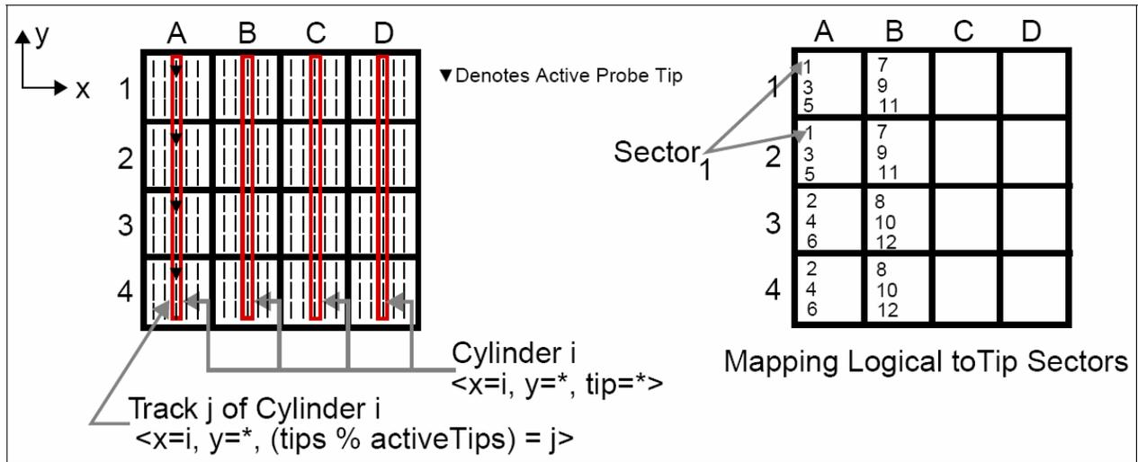
**Figure 2: Cylinders, Tracks, and Sectors [10]. All the columns with the same X coordinate form a cylinder. Track j consists of tip sectors within a cylinder that are accessible by the concurrently active tips. In this example, tip A1, A2, A3, A4 can be active simultaneously and activeTips = 4. The tips are linearly indexed (A1 = 0, B1=1, C1=2, etc.). Each logical sector, shown on the right side, is striped across two tip sectors.**
