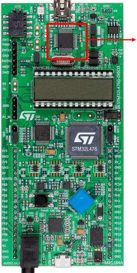
Integrated ST-Link/V2 programming and debugging tool
