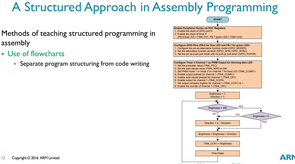
Diming LED by using timer PWM output
