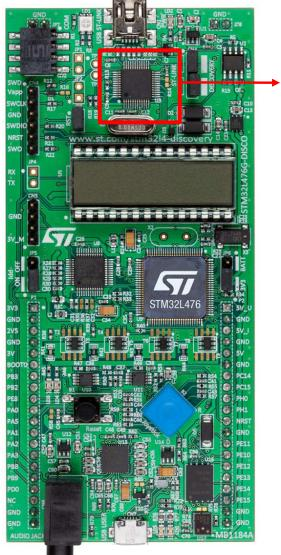
Integrated ST-Link/V2 programming and debugging tool
