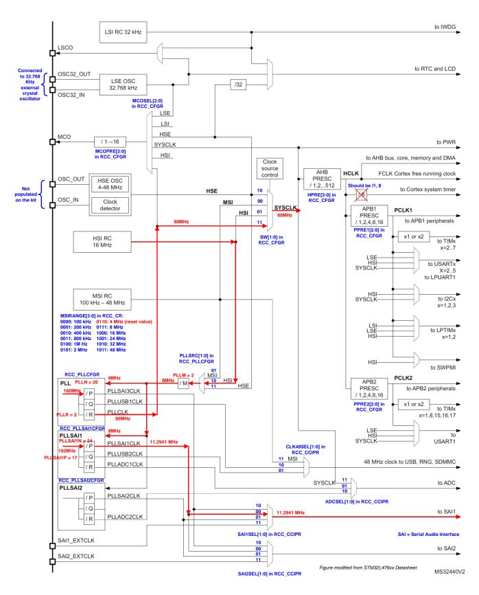
Diagram configuring SYSCLK as 80 MHz and SAI to 11.2941 MHz. (SAI is not used in this lab)
