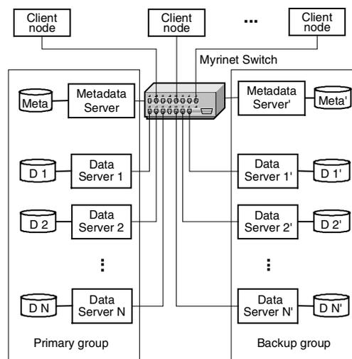
Figure 1. Block Diagram of CEFT-PVFS.
