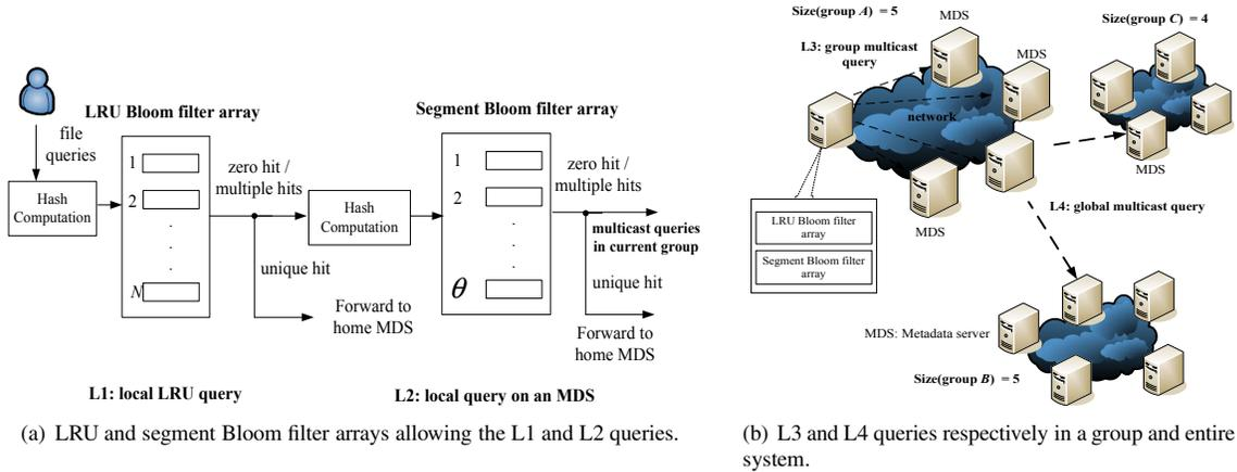
**Figure 1. The group-based HBA architecture allowing the multi-level query.**
