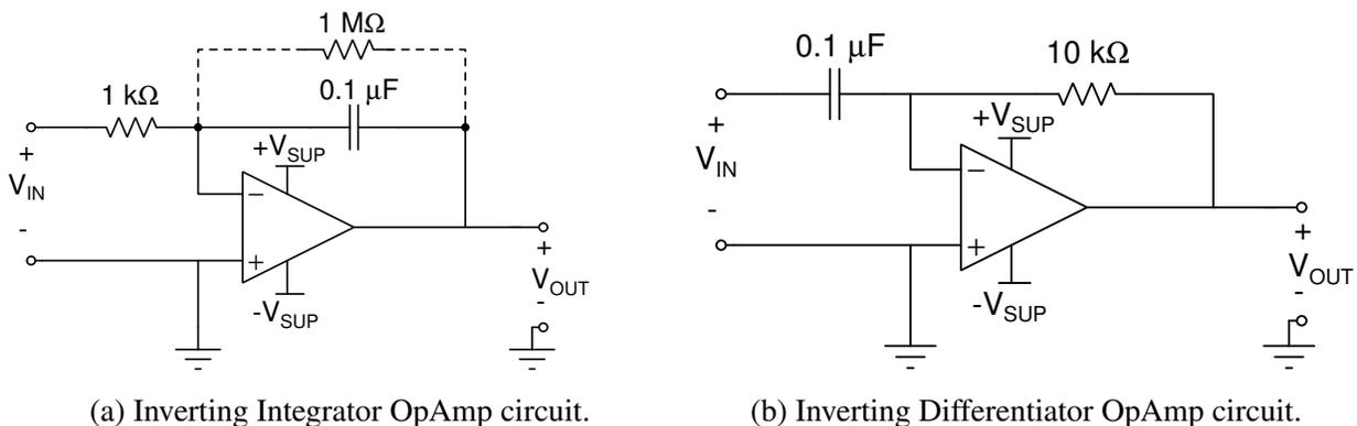
Figure 2: Inverting Integrator and Inverting Differentiator OpAmp Circuits
