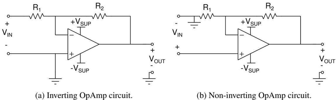
Figure 1: Inverting and Non-inverting OpAmp Circuits
