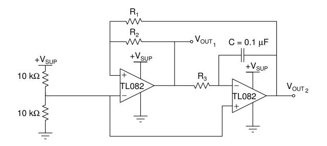
• A Schmitt trigger hooked to an inverting integrator with feedback.
