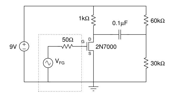
2. Hook up to the function generator with a triangle wave,
