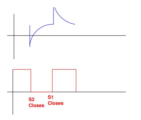
With switch open (output 9V), capacitor charges to 9V on one side, 3V on other. When switch closes (output 0V), capacitor voltage now in reverse, 0 and -6V.
