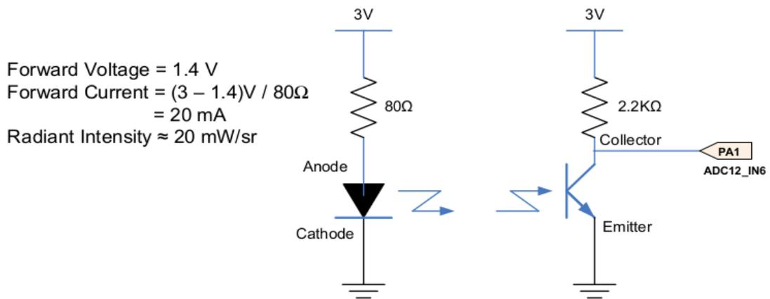
Figure 4: Connection diagram.
