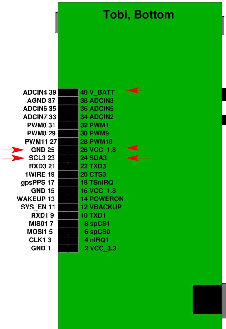
Figure 1: 40-pin header output on Tobi board
