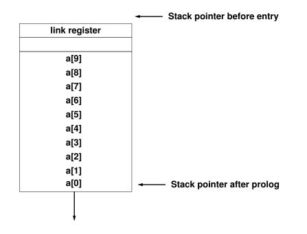
A value written to a[11] overwrites the saved link register. If you can put a pointer to a function of your choice there you can hijack the code execution, as it will be jumped to at function exit.
