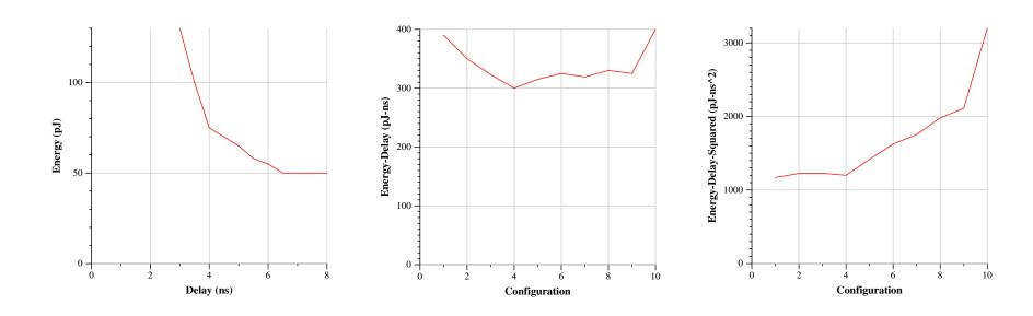
Roughly based on data from "Energy-Delay Tradeoffs in CMOS Multipliers" by Brown et al.
