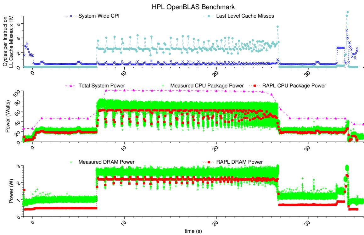
Figure 5: HPL OpenBLAS Benchmark. Yes, anonymous reviewer #2, the CPU line crosses over the total line; this can happen when your total power measurement is only sampling at 1Hz.
