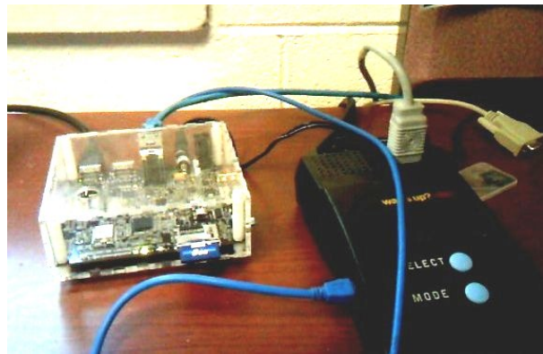
Figure 1: WattsUpPro hooked to an ARM development board. TODO: get a better picture.
