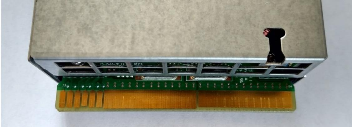
Figure 3.6: HP Common Slot Power Supply Contacts
