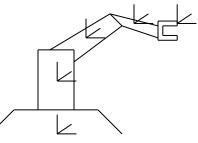
Sometimes we think of the relation between two frames as a sequence of motion to get from one pose to the other. In this case the frames OXYZ (fixed reference system) and OUVW (moving system) are initially aligned:
