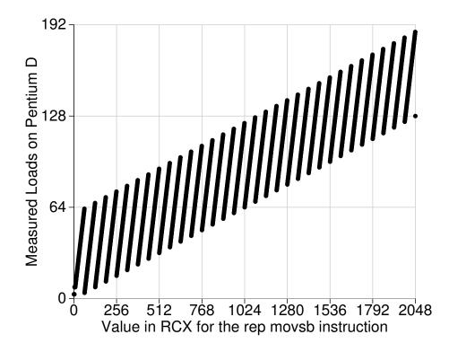
Figure 1: On Pentium D, the retired loads event shows unusual behavior with rep movs string instructions. The observed count is related to 64-byte chunks being moved with individual moves for the remainder: (floor(reps/64) \* 4) + (reps%64).
