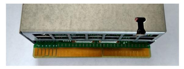
Figure 3.6: HP Common Slot Power Supply Contacts
